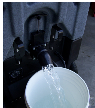
Drain water from Recovery Tank
