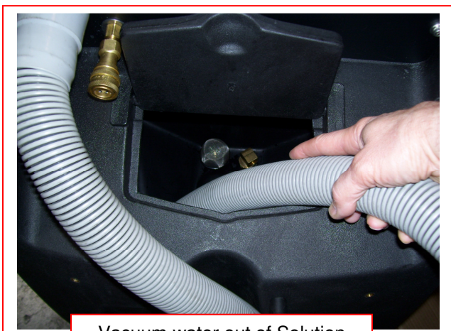
Vacuum water out of Solution Tank
