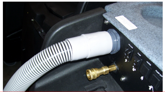
Vacuum Connection with standard barb and vinyl cuff
