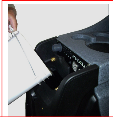
Pour appropriate amount of hot water into solution tank
